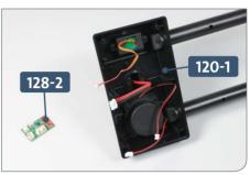
Insert the connector for the speaker cable 124-1 and cable 127-5 into the other two sockets, as pictured.
