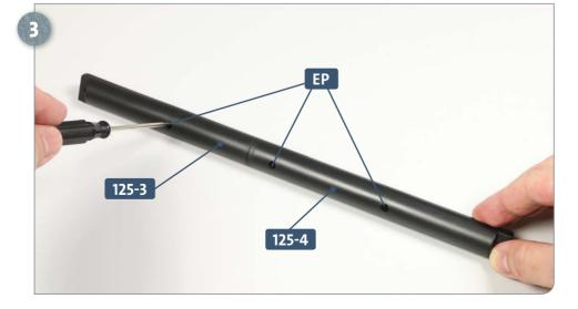
Join the four sections of the longitudinal beam together using the three **EP** screws through the holes of the two lower sections, **125-3** and **125-4**.
