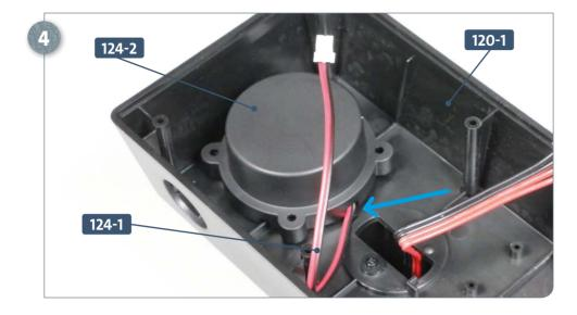
Place the bracket **124-2** over the speaker **124-1**, positioning its four tabs over the screw holes in the body of the stand **120-1**. Make sure that the speaker cable is routed through the recess in the bracket, which is indicated by the arrow.
