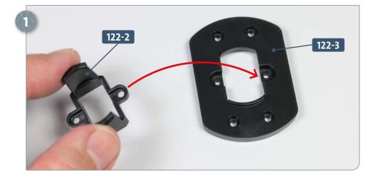
Place the lower half of the front bracket 122-3 on your work surface. Take the connector 122-2 and fit the two side tabs into the recesses of the bracket, as indicated by the arrow.
