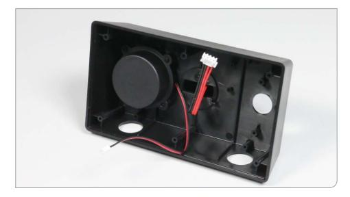
The speaker has now been installed in the aft part of the stand.
