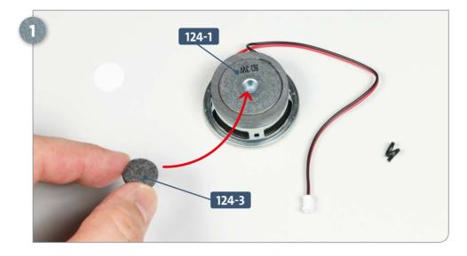
Take the speaker **124-1** and remove the tie from the cable. Remove the backing from the pad **124-3** and fit it onto the speaker, as indicated. See also the next step.
