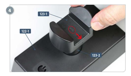
Fit the support column **123-2** onto the main body of the forward stand **122-1**. Make sure that the arrow embossed into the bracket **123-1** (circled) points in the direction shown in the photo.
