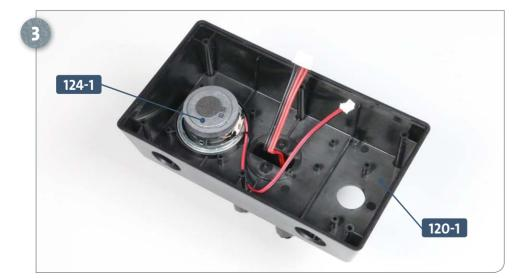
Place the aft stand **120-1** upside down on your work surface. Fit the speaker **124-1** into the perforated, ribbed area of the stand, as pictured.
