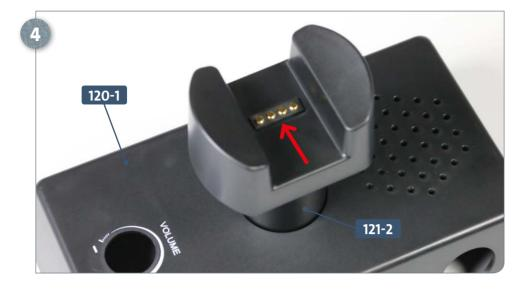
Feed the contact cable **121-3** through the rectangular opening in the body of the aft stand **120-1** (see inset photo). Place the support column **121-2** on the stand. Make sure that the opening for the contacts (see arrow) is not in the centre of the bracket, but aligned as shown in the photo.
