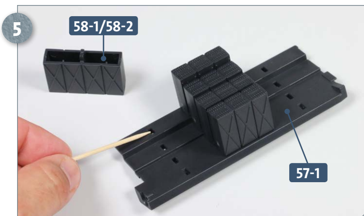
Take one of the battery cells 58-1/58-2 and the installation rail 57-1 , oriented as shown. Add some glue inside the slot indicated by the cocktail stick in the image above.
