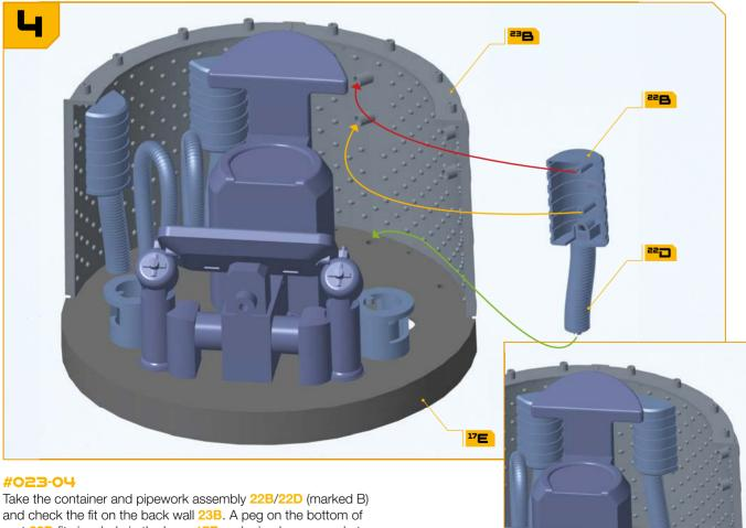
part 22D fits in a hole in the base 17E and raised screw sockets in part 22B fit into screw holes in part 23B (arrows).
