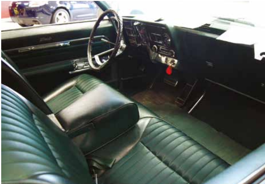
Left: With no transmission tunnel, there was extra space for the driver.
