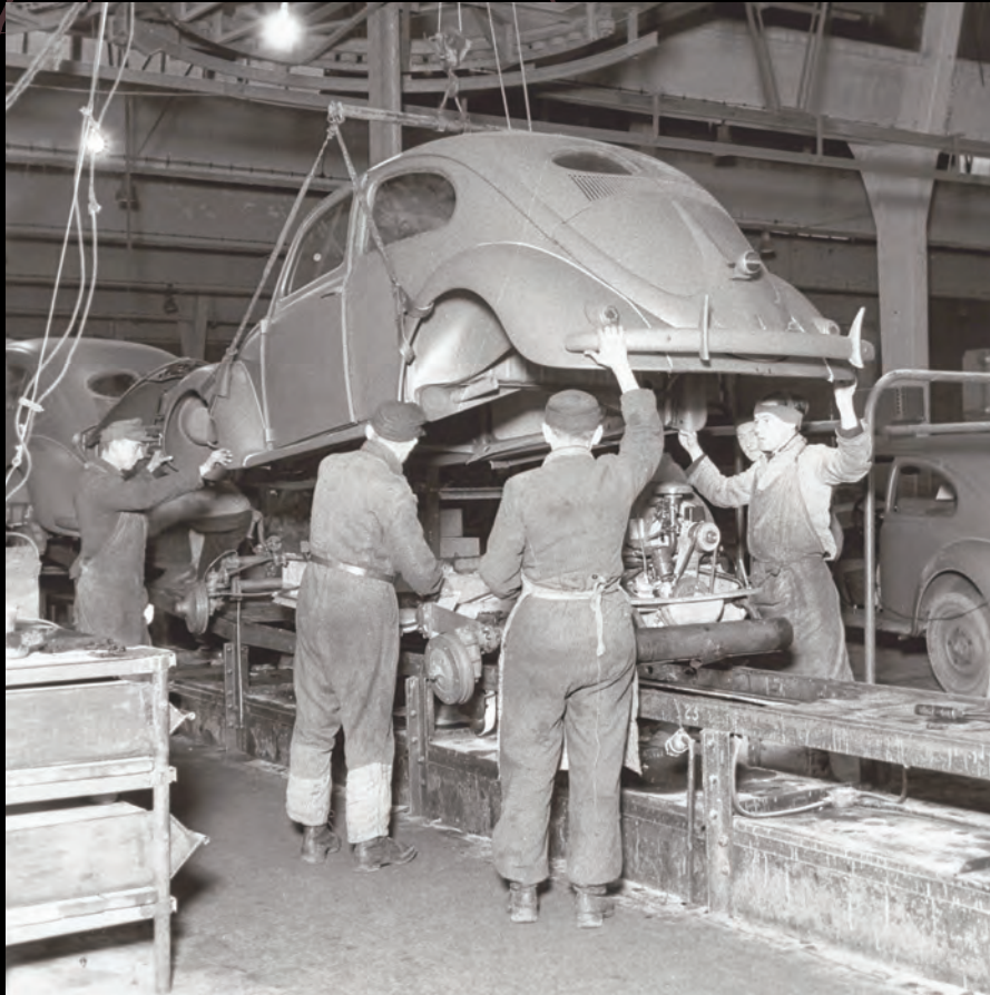
German workers lower a beetle body on to the chassis in the Wolfsburg plant factory in 1946.
